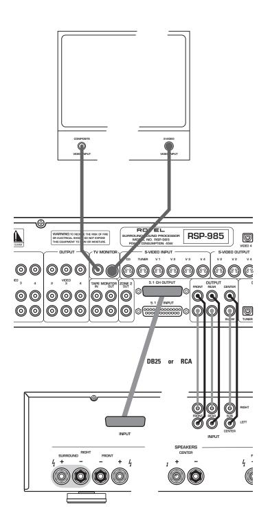
Figure 4 - RCA Source Connections
